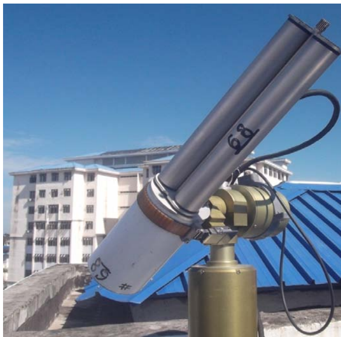
Fig. 3: AERONET sun photometer placed on the roof of the academic building at UiTM Penang
