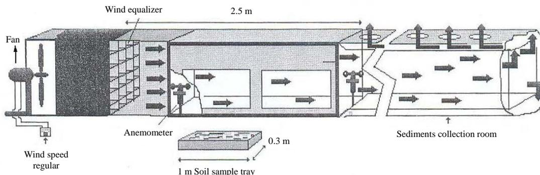
Fig. 1: Schematic diagram of the wind tunnel structure
