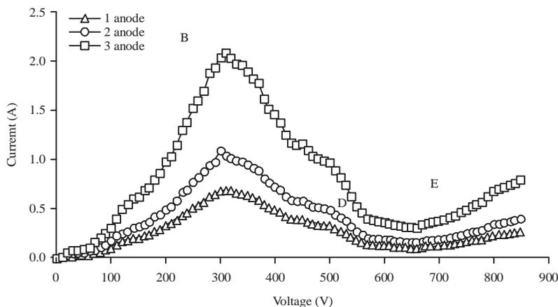
Fig. 4: Characteristic of m-CGDE current-voltage with different anode, electrolyte: 0.02 M KOH, anode material: Tungsten
