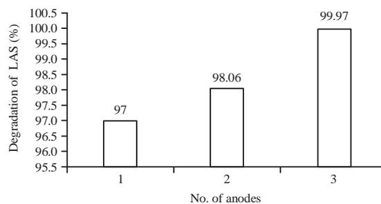
Fig. 7: Percentage degradation of LAS on variation of the number of anodes within 30 min process, electrolyte: KOH 0.02 M, [LAS] initial: 100 ppm, anode: Tungsten, voltage: 700 V, stirrer speed: 500 rpm
