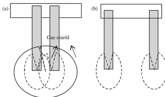
Fig. 8(a-b): Anodes distances, (a) Close anodes and (b) Distant anodes
