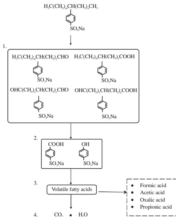
Fig. 2: Scheme of LAS Degradation<sup>4</sup>
