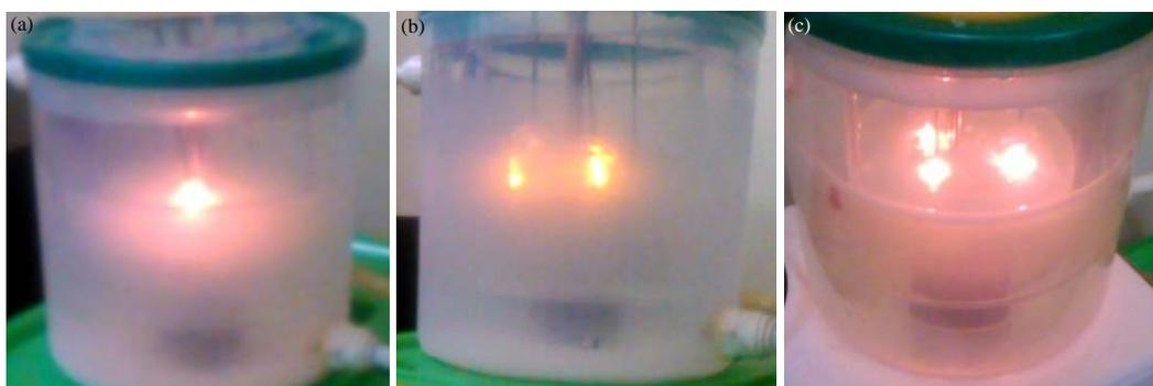
Fig. 5(a-c): Visualization of plasma formation with different number of anodes, (a) 1 anode, (b) 2 anodes and (c) 3 anodes, electrolyte: 0.02 M KOH, voltage: 700 V, anode material: Tungsten
