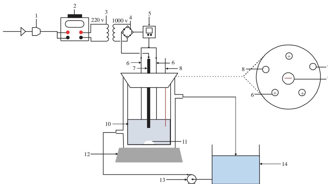
Fig. 3: Schematic diagram of CGDE triple-anode reactor for LAS waste treatment<sup>2</sup>, 1: MCB, 2: Slide regulator, 3: Trafo, 4: Diode bridge, 5: Multi-meter, 6: Anode, 7: Cathode, 8: Thermometer, 9: Sample hole, 10: LAS waste, 11: Magnetic stirrer, 12: Stirrer, 13: Pump and 14: Cooling water
