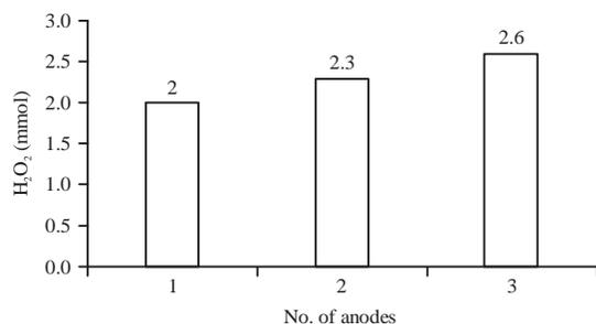
Fig. 6: H<sub>2</sub>O<sub>2</sub> level comparison on variation of the number of anodes. Within 30 min process, electrolyte: KOH 0.02 M, anode: Tungsten, voltage: 700 V, stirrer speed: 500 rpm
