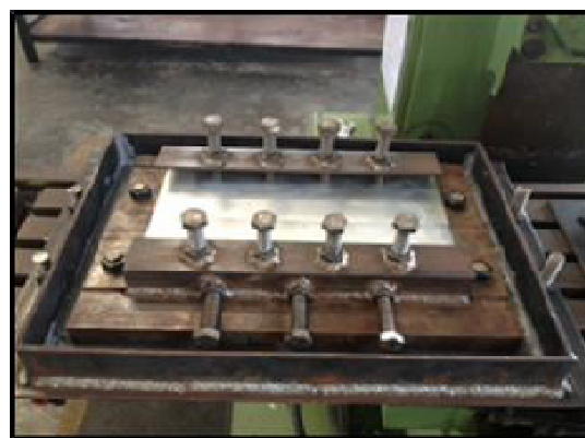
Fig. 4: A complete jig and tank with the specimen
