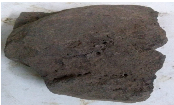
Fig. 5: Gravel size LD slag (photograph taken at Bokaro Steel Plant, Jamshedpur, India)
