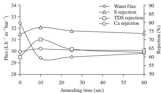
Fig. 5: Effect of thermal annealing time on the membrane performance
