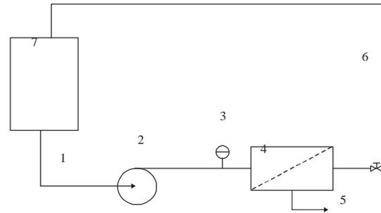
Fig. 1: Dead-end filtration cell, 1: Feed stream, 2: Feed pump, 3: Pressure gauge, 4: Membrane module, 5: Permeate, 6: Retentate and 7: Feed tank
