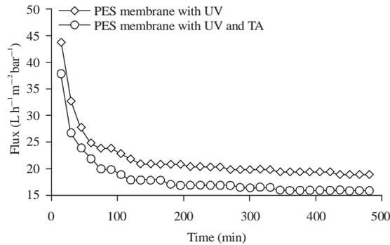
Fig. 8: Modified PES membrane stability in term of flux
