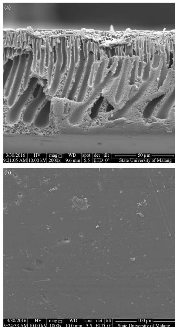
Fig. 6(a-b): SEM images of membrane morphology (a) Cross-section and (b) Surface section
