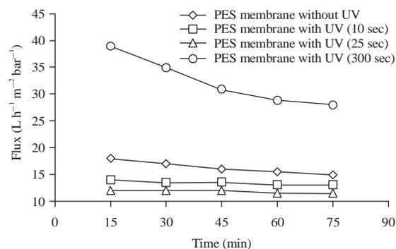
Fig. 2: Effect of UV irradiation on the membrane flux
