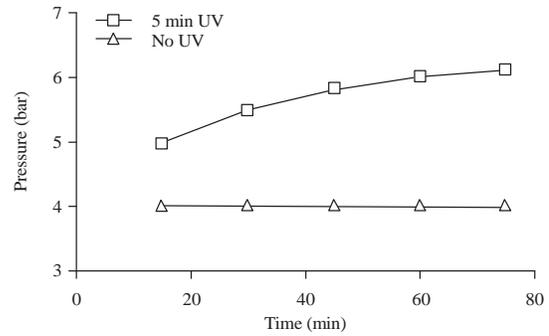
Fig. 3: Operation pressure of produced water treatment with UV irradiation membrane
