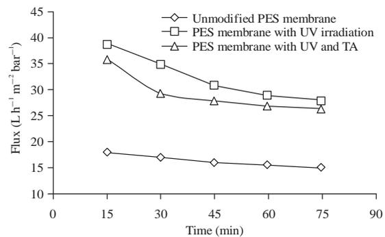
Fig. 4: Effect of combination treatment on the membrane flux
