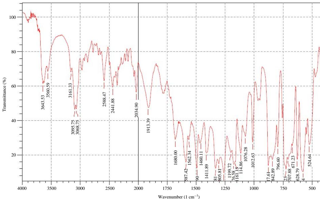
Fig. 7: FTIR result of PES membrane 19% weight, 5 min UV, 10 sec thermal annealing
