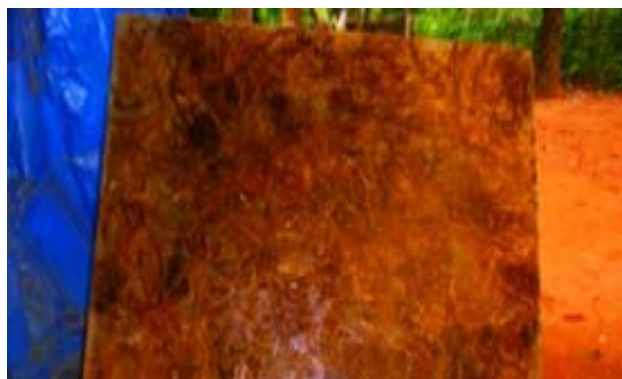
Fig. 1: Fabricated bamboo fibre reinforced composites
