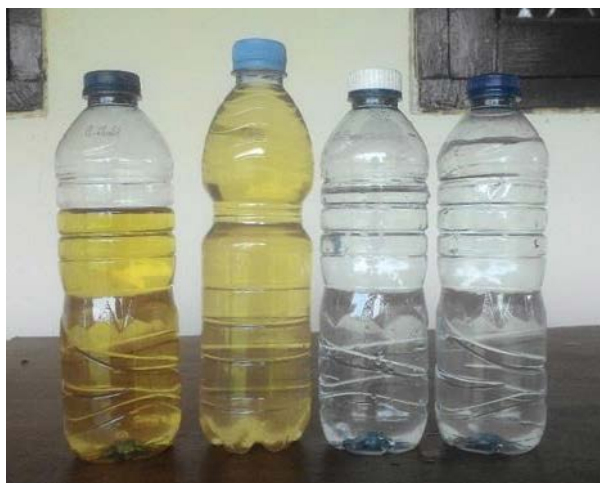
Fig. 4: Peat water sample before treatment (brownish) and after treatment with coagulants and slow sand filters (limpid)
