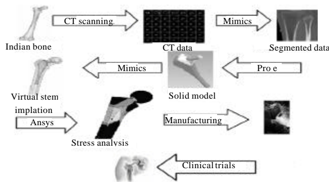
Fig. 1: Work flow diagram for designing Hip prosthesis
