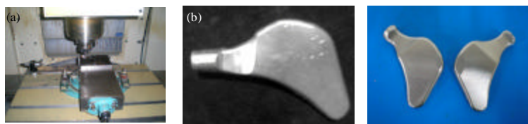
Fig. 7(a-b): (a) Implant machining and (b) photographs of newly designed short femoral stem
