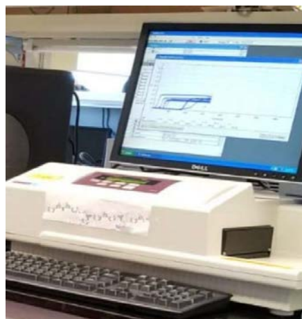
Fig. 2: Fluorescence microplate reader connected to a computer workstation for acquisition and analysis of clot-based coagulation assay data
