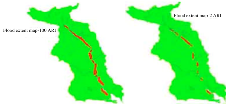
Fig. 5: Water level modeling with InfoWorks in Skudai River from Sedenak Plantation area (upstream) to Danga Bay (downstream)-100 ARI
