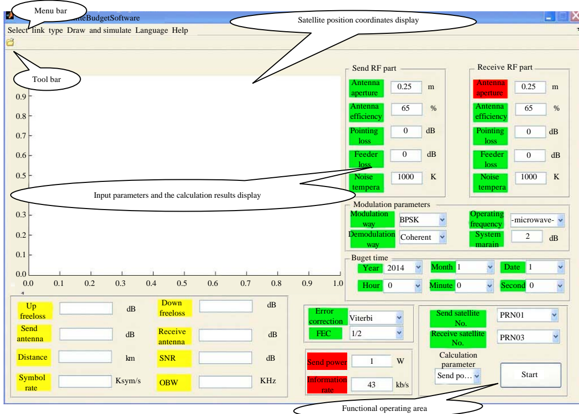
Fig. 3: Microwave link budget interface design plan
