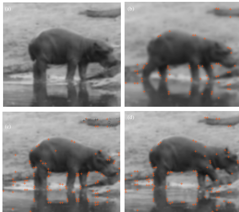
Fig. 2(a-d): Results of corner detector (a) 1st, (b) 2nd, (c) 3rd and (d) 4th frame, respectively
