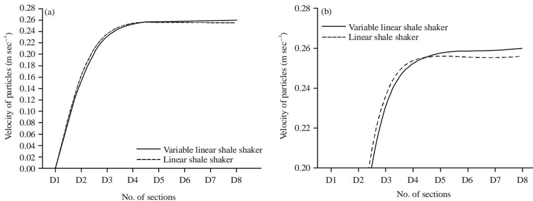
Fig. 9(a-b): Conveyance velocity of particles at different sections of the screen, particles at every section and (b) Velocity of particles at main section
