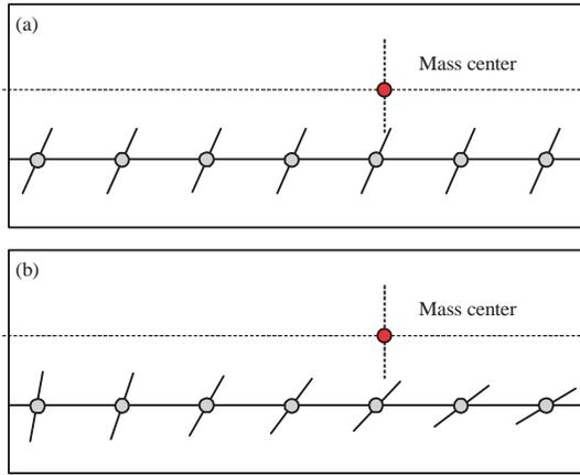
Fig. 2(a-b): Motion trajectory of key points on screen deck, (a) Linear trajectory and (b) Variable linear trajectory
