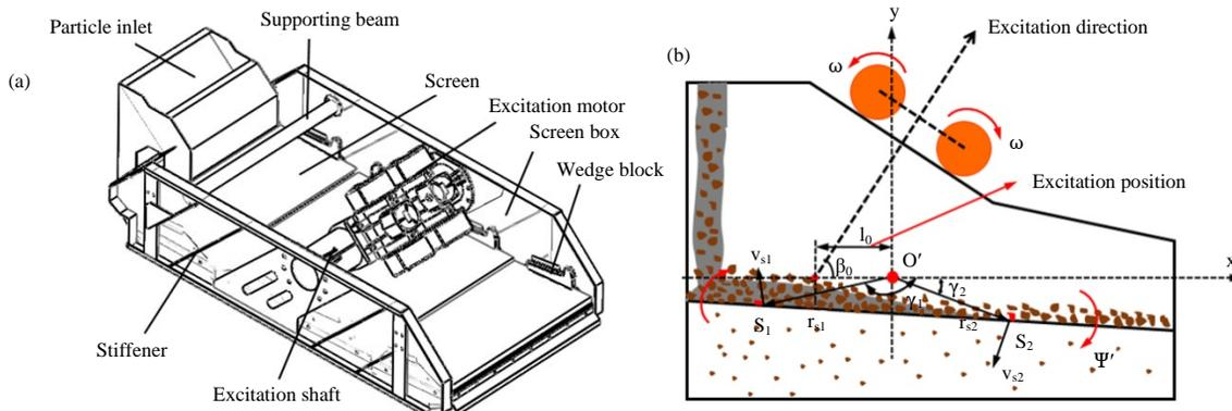
Fig. 1 (a-b): Motion analysis diagram of screenbox system, (a) Actual structure of shale shaker and (b) Schematic diagram of shale shaker
