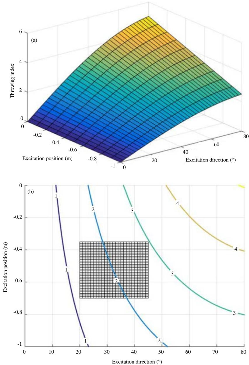
Fig. 6(a-b): Distribution of throwing index at outlet, (a) Distribution of throwing index and (b) Projection figure of contour line
