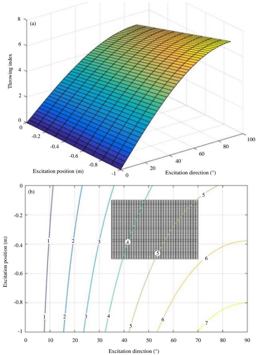
Fig. 5(a-b): Distribution of throwing index at inlet, (a) Distribution of throwing index and (b) Projection figure of contour line
