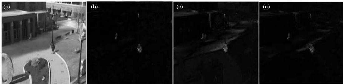
Fig. 7(a-d): Contrast of detection effect in case of outdoor lighting changes, (a) Input image, (b) Our algorithm test results, (c) Gaussian mixture algorithm test results and (d) Codebook algorithm test results
