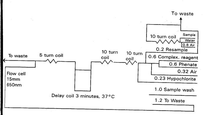
Fig. 1: AutoAnalyzer Manifold for Determining NH<sub>4</sub>-N
