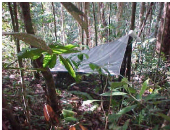
Fig. 1: One of the Malaise trap used showing the collecting insect bottle at one end of its raised roof.
