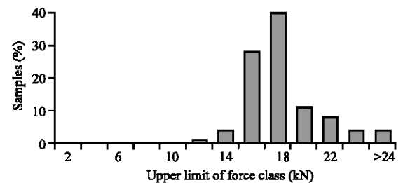
Fig. 7: Frequency distribution of the moldboard plow draft forces (Nafferton Farm)
