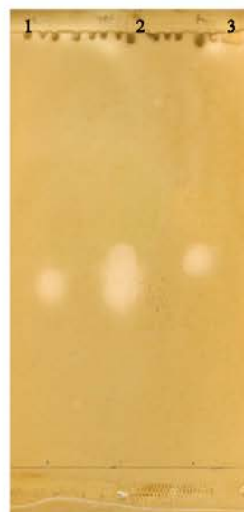
Fig. 5: Enzyme activity assay figured by Thin Layer Chromatography (TLC), Lane 1: standard mannitol, Lane 2: sample of the enzyme assay with fructose as a substrate, Lane 3: standard of fructose
