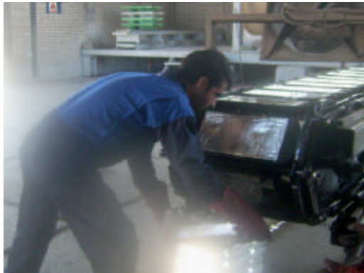
Fig. 2: A worker is lifting a zinc bar of 30 kg with bent back
