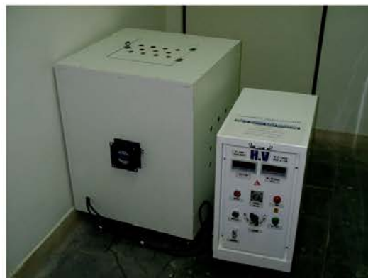
Fig. 1: Electromagnetic field producer system
