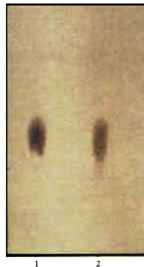
Fig. 3: Paper chromatography of extracted Des. from S. pilosus (ATCC 19797) (2) and standard Desferal (1). Rfs are 0.457 and 0.462, respectively. These results show that the produced Des in S. pilosus is B-type
