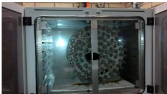
Fig. 2: Fermentation chamber of «Hohenheim» biogas yield testing system
