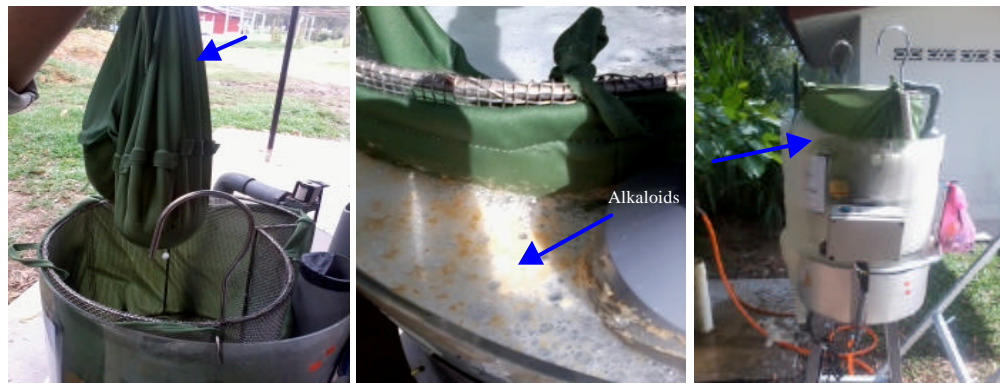
Fig. 5: Machine basket with fabric filter and the bubbles alkaloid during machine operation
