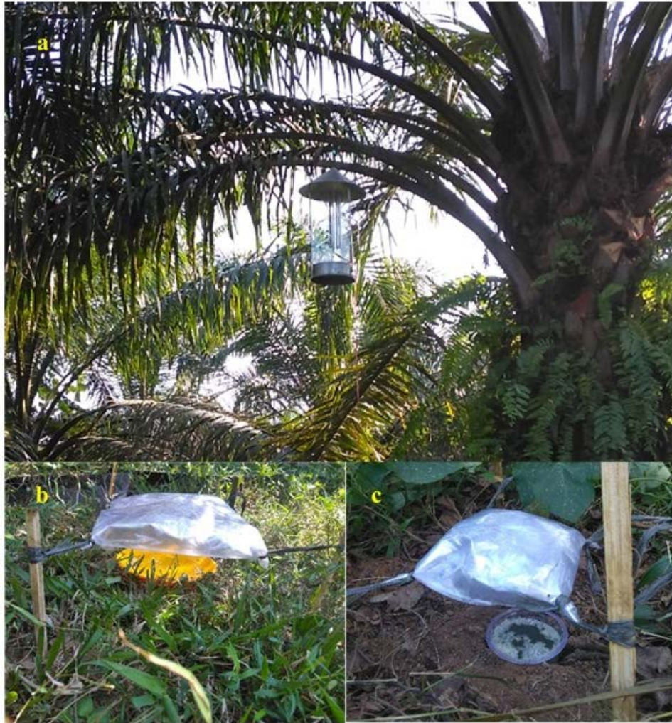
Fig. 3(a-c): The traps used to collect arthropod samples in immature and mature oil palm plantations: (a) Light trap, (b) Yellow pan trap and (c) Pitfall trap
