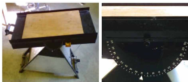
Fig. 2: The device for determining coefficient of static friction
