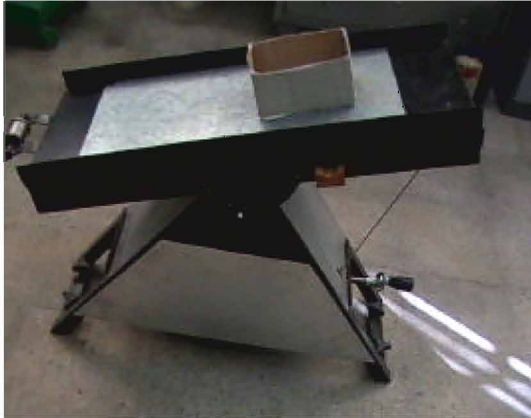
Fig. 1: Apparatus for measuring static coefficient of friction.
