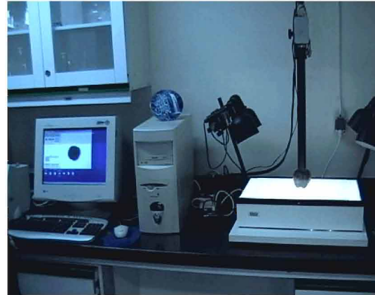
Fig. 2: Area Measurement System-Delta Tengland for measuring projected area of apples.
