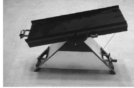
Fig. 2: Apparatus to determine coefficient of static friction.
