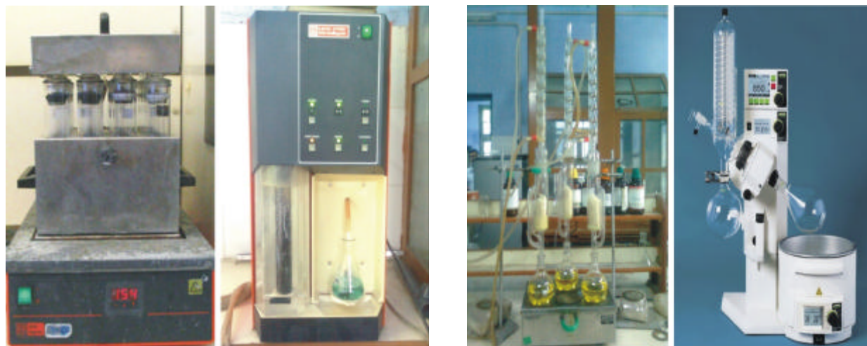
Fig. 3: Images of (A) Digester, (B) Micro Kjeldahl's apparatus, (C) Soxhlet extractor (D) Rotary Evaporator
