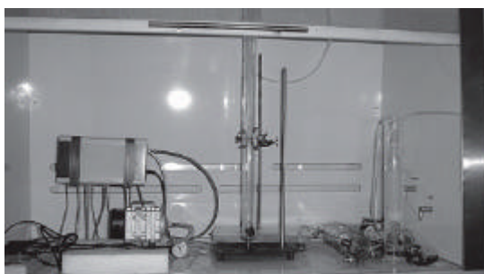
Fig. 3: Experimental set-up for ozone COD and colour removal
