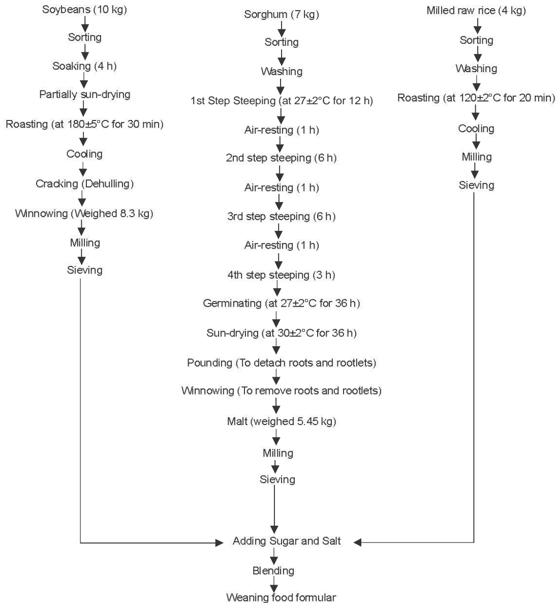
Fig. 1: Production of complementary food formulations from mixtures of improved rice cultivars and soybean (Adapted from Badau et al. (2005) with slight modification)
