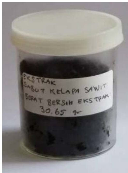
Fig. 1: Extract from oil palm fronds using ethanol as a solvent
