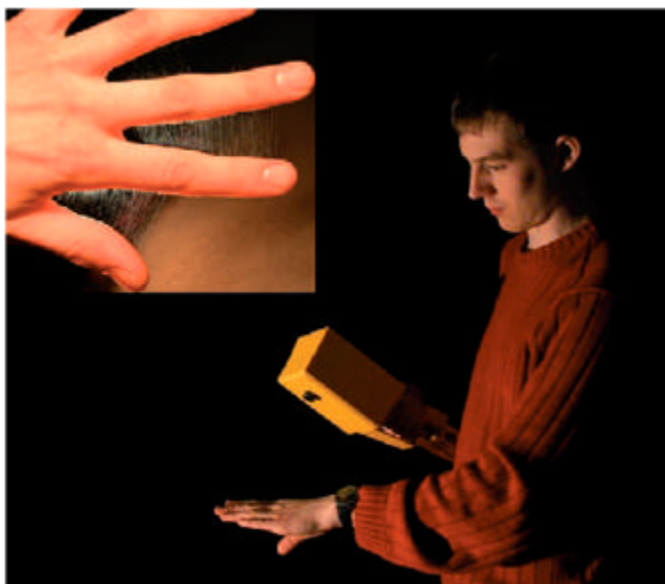
Fig. 9: Handheld device for the electrospinning of wound dressings. Inset: PEO fibers electrospun from aqueous solution onto a hand (Greiner and Wendorff, 2007)
