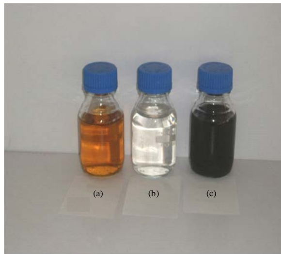
Fig. 2(a-c): Green synthesis of AgNPs, (a) Aqueous leaf extract of T. involucrata , (b) 20 mM aqueous \text{AgNO}_3 and (c) Colour changed from yellowish to black after adding 20 mM aqueous \text{AgNO}_3
