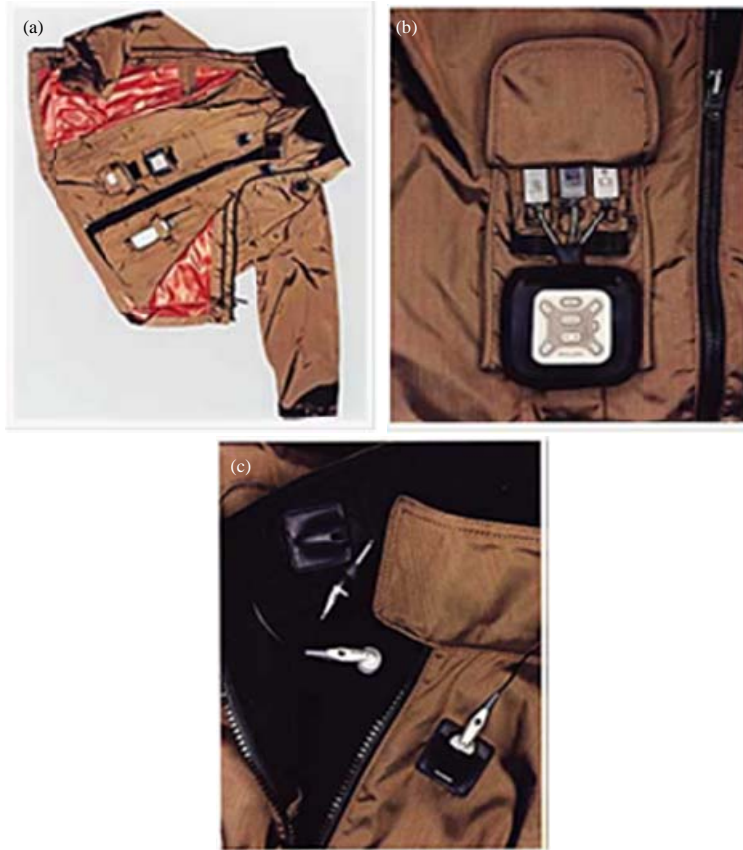
Fig. 1(a-c): Mooring jacket with (a) Communication systems, (b) Speakers and (c) Microphones
