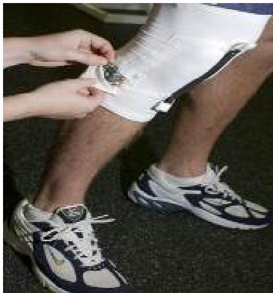
Fig. 17: Intelligent knee sleeve with microcontroller driven alarm tone
