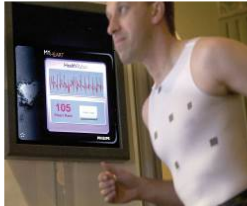
Fig. 10: On-body sensors and electronics for monitoring vital body signs - a garment with textile ECG electrodes developed by the MyHeart project to prevent heart failure. (Source: Philips)
