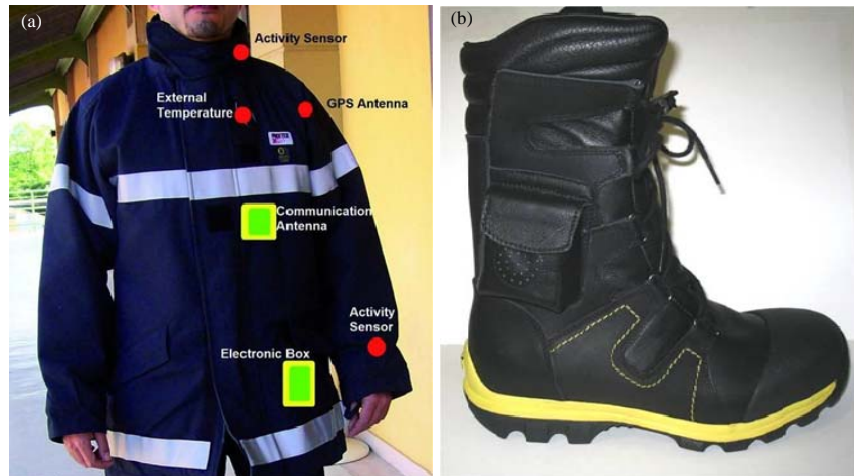
Fig. 16(a-b): (a) Fire fighter outer garment and (b) Boot with gas sensor
