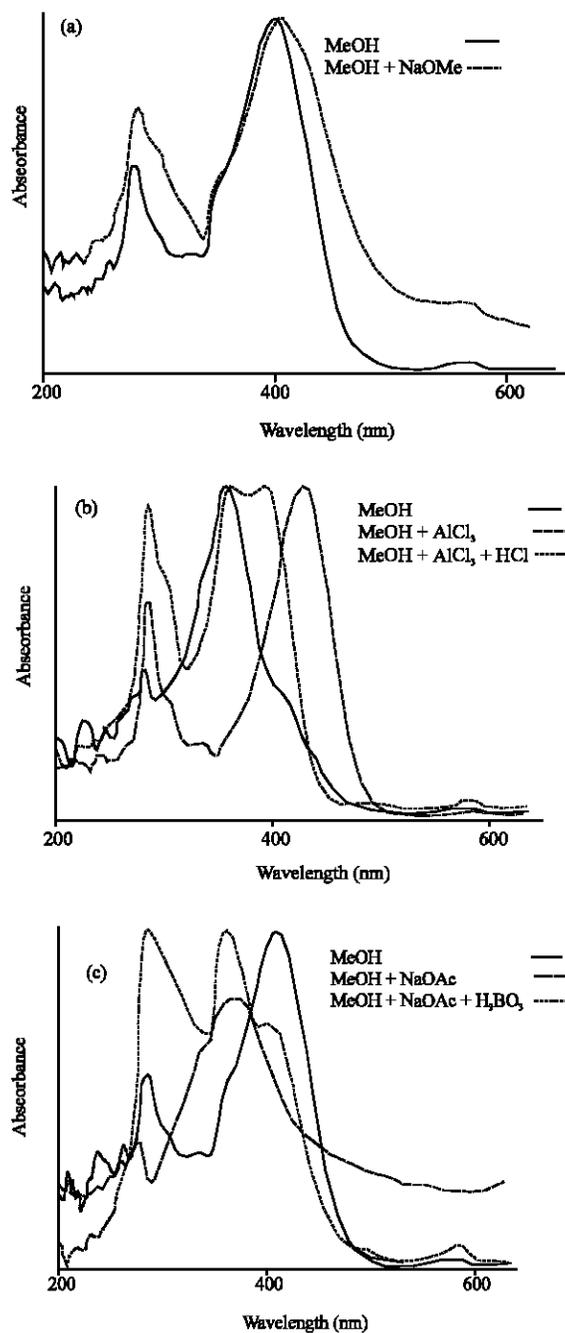
Fig. 5: UV/Vis absorption spectra of compound G-II in (a) MeOH and MeOH/NaOMe, (b) MeOH, MeOH/AlCl<sub>3</sub> and MeOH/AlCl<sub>3</sub>/HCl and (c) MeOH, MeOH/NaOAc and MeOH/NaOAc/H<sub>3</sub>BO<sub>3</sub>
