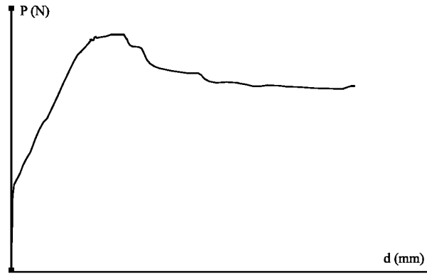
Fig. 5: Graph of load (P) against displacement (d) for 10 layers silk fibre
