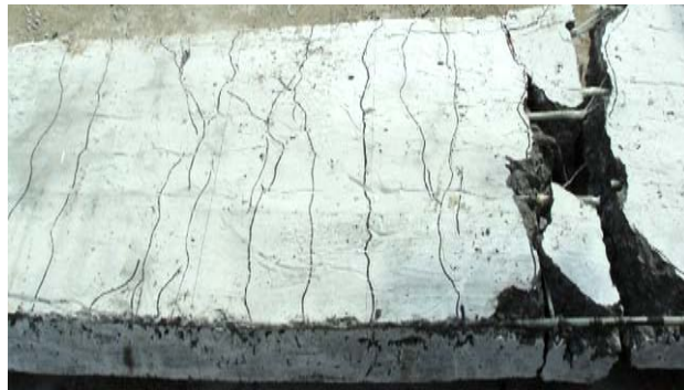
Fig. 18: Crack pattern of plain GFRP reinforced slab
