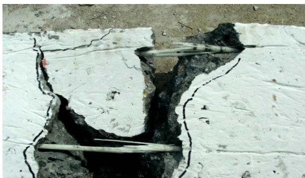
Fig. 14: Rupture of GFRP reinforcement
