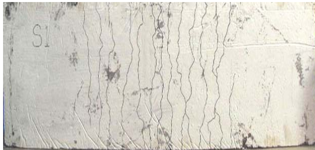
Fig. 16: Crack pattern of conventional slab
