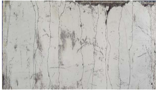
Fig. 17: Crack pattern of sand coated GFRP reinforced slab
