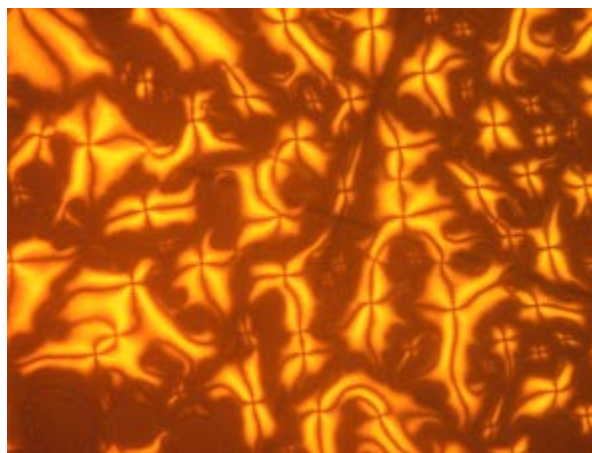
Fig. 2: Optical photomicrograph of compound 4 at 160.2^{\circ}\text{C} on cooling from the isotropic liquid
