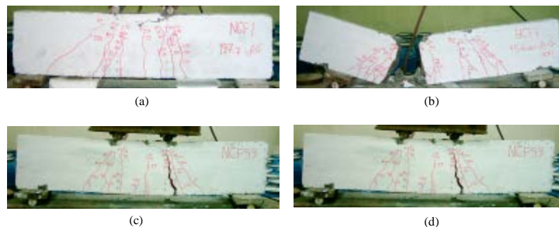
Fig. 7: Methods of disruption of some of the specimen beams; (a) NCF1, (b) HCF7, (c) NCF59, (d) HCFS13
