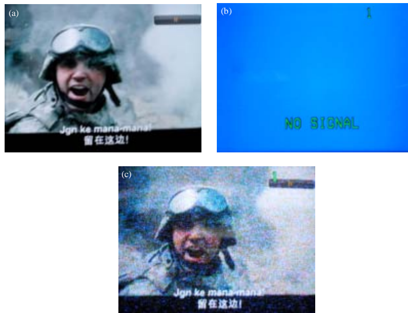
Fig. 8: One failure case where signals send to protection line. (a) Received from transmitter, (b) Received from working line and (c) Received from protection line
