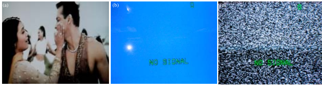
Fig. 9: Two failure cases where both working and protection are failure. (a) Received from transmitter, (b) Received from working line and (c) Received from protection line
