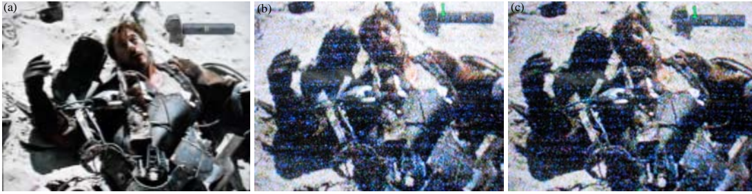
Fig. 6: Signals send to both working and protection lines. (a) Received from transmitter, (b) Received from working line and (c) Received from protection line
