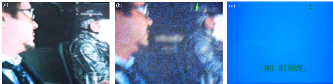
Fig. 7: Normal condition where signals send to working line. (a) Received from transmitter, (b) Received from working line and (c) Received from protection line
