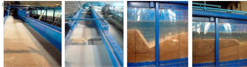
Fig. 4: The variation of bed due to migration of the trapezoidal pit
