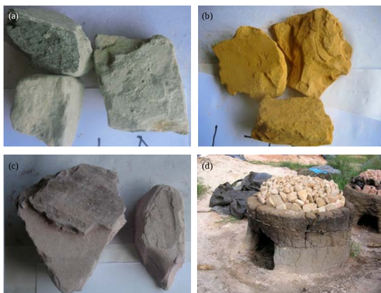
Fig. 1(a-d): Photography of (a) Green clay of Anyama (AVA), (b) Yellow Lokpo (LJFF), (c) Purple Lokpo (LVF) and (d) White Lokpo (LBF) in a traditional oven for thermal treatment
