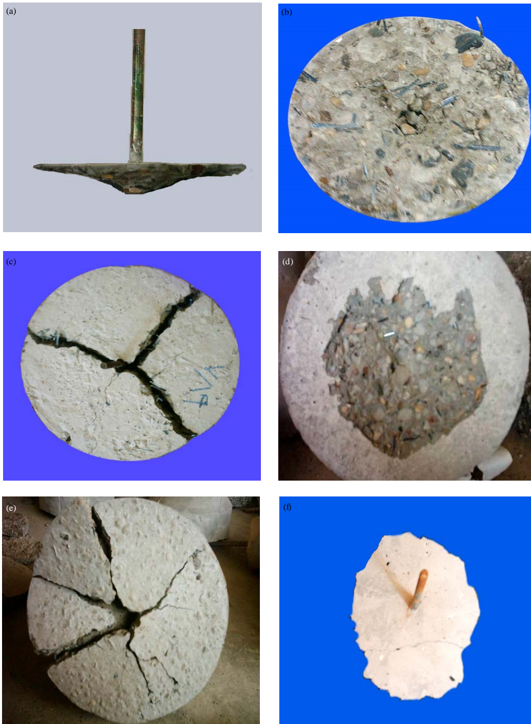
Fig. 2(a-f): Failure patterns of some specimens (a) f'_c = 30 MPa, h_{ef} = 25 mm, d_b = 8 mm, V_f = 0 , (b) f'_c = 27.4 MPa, h_{ef} = 37.5 mm, d_b = 10 mm, V_f = 12\% , L_f = 32 mm, (c) f'_c = 34.5 MPa, h_{ef} = 62.5 mm, d_b = 10 mm, V_f = 0.8\% , L_f = 16 mm, (d) f'_c = 45 MPa, h_{ef} = 37.5 mm, d_b = 12 mm, V_f = 0.8\% , L_f = 32 mm, (e) f'_c = 53 MPa, h_{ef} = 50 mm, d_b = 10 mm, V_f = 1.2\% , L_f = 32 mm and (f) f'_c = 58 MPa, h_{ef} = 25 mm, d_b = 10 mm, V_f = 0
