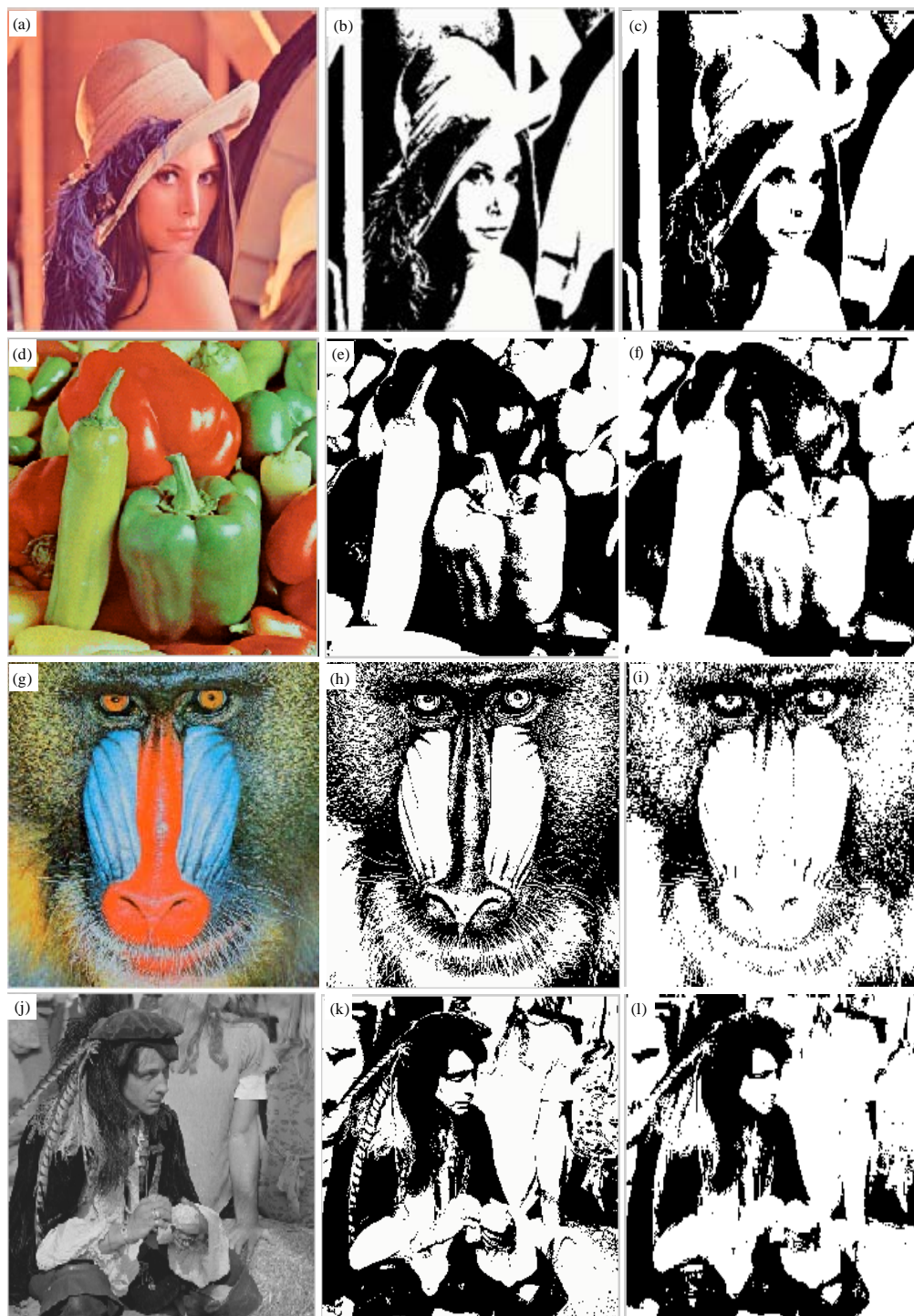
Fig. 8(a-l): Comparison of experimental results of PSO segmentation given MATLAB and XSG tool, (a) Lenna, (d) Peppers, (g) Mandrill, (j) Hunter, (b, e, h, k) Experimental results of PSO segmentation using MATLAB, (c, f, i, l) Experimental results of PSO segmentation using XSG
