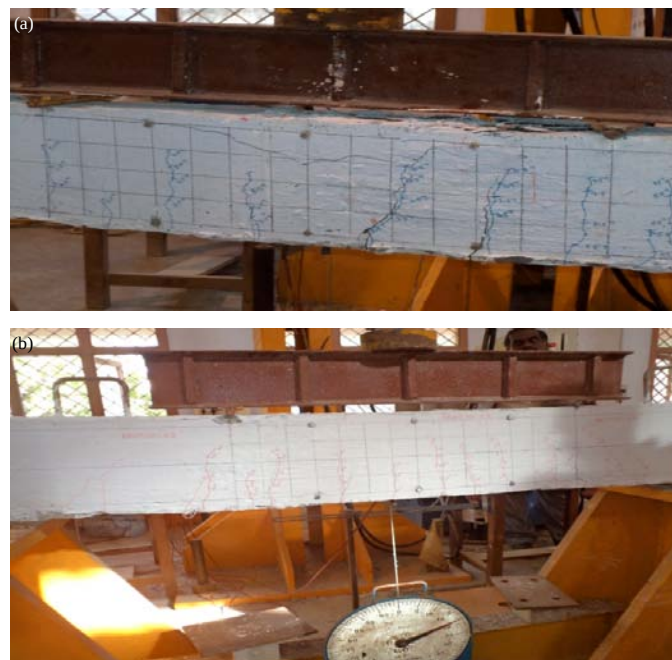
Fig. 4(a-b): (a) Details of crack propagation for a beam with control concrete and (b) Details of crack propagation for a beam with high volume fly ash recycled aggregate
