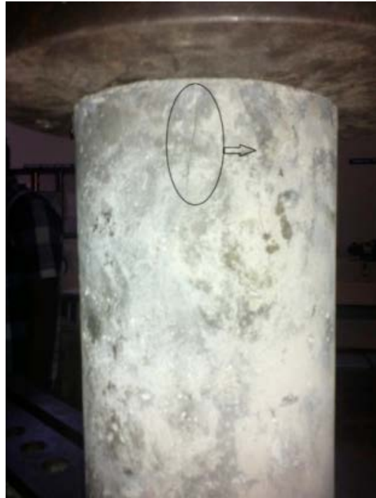
Fig. 5: Initiation of crack in cylinder specimen
