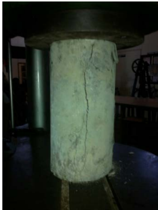
Fig. 6: Failed specimen after ultimate load
