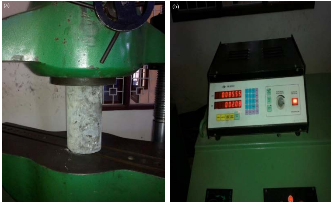
Fig. 4(a-b): (a) Load setup for cylinder specimen and (b) Automatic data acquisition system
