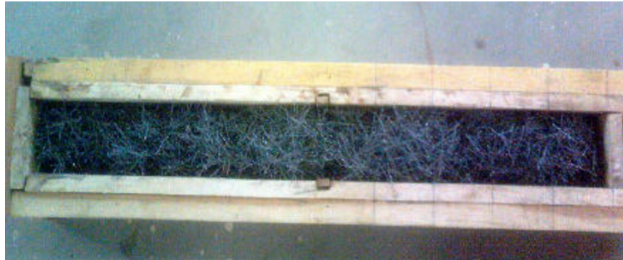
Fig. 1: Steel fibers preplaced in the mould before pouring of slurry
