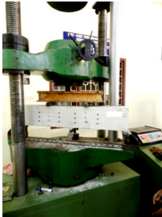
Fig. 3: Loading arrangement of the beam specimen before testing
