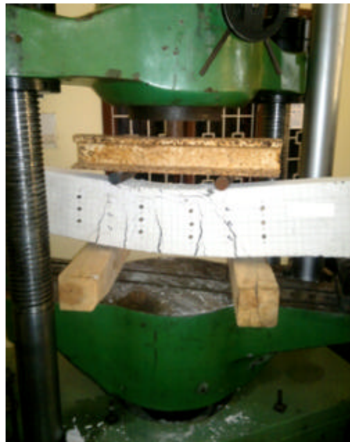
Fig. 6: Failure pattern of the beam specimen after testing
