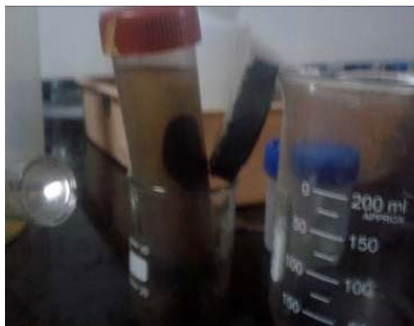
Fig. 2: Pathogen isolation using Ch-MNPs by placing external magnet near test tube
