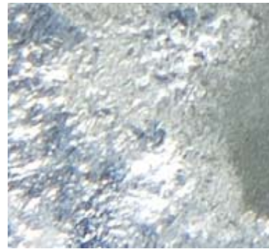
Fig. 2: Solder test after electroplating with persulfate as descale 10
