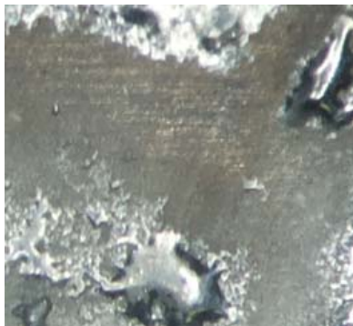
Fig. 1: Solder test after electroplating with standard surface cleaning 10
